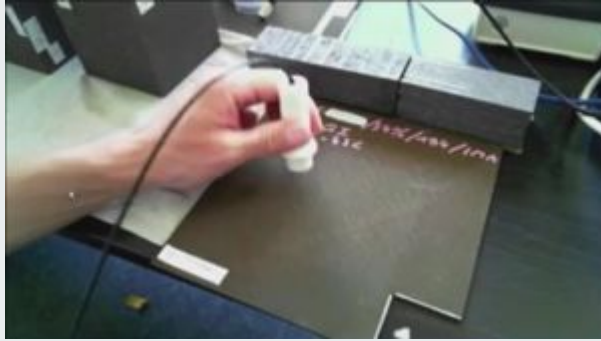
Measurement electrical conductivity of carbon composite materials (CFRP)
